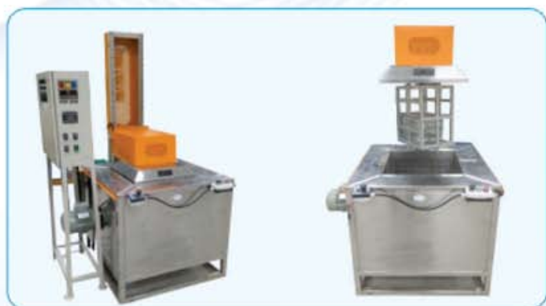
Auto basket clamping inside the work chamber
